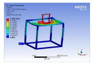
Figure 3: Total deformation in frame
