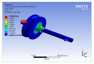
Figure 4: Equivalent stresses acting in rollers
