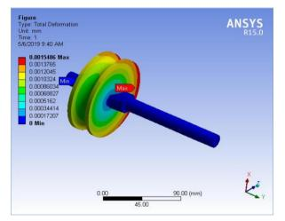
Figure 5: Total Deformation in rollers
