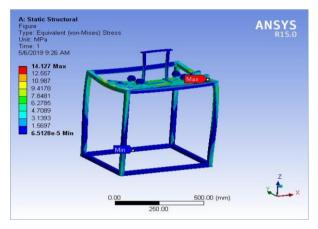
Figure 2: Equivalent stresses acting on frame
